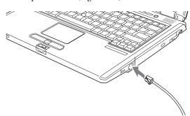
Figure 4-15. Connecting a Modem
